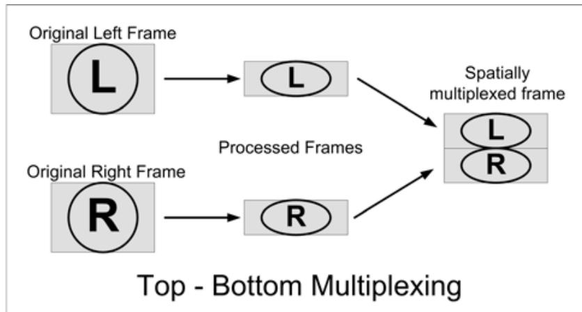
**Figure 5.1** Top-Bottom Multiplexing<sup>1</sup>.
