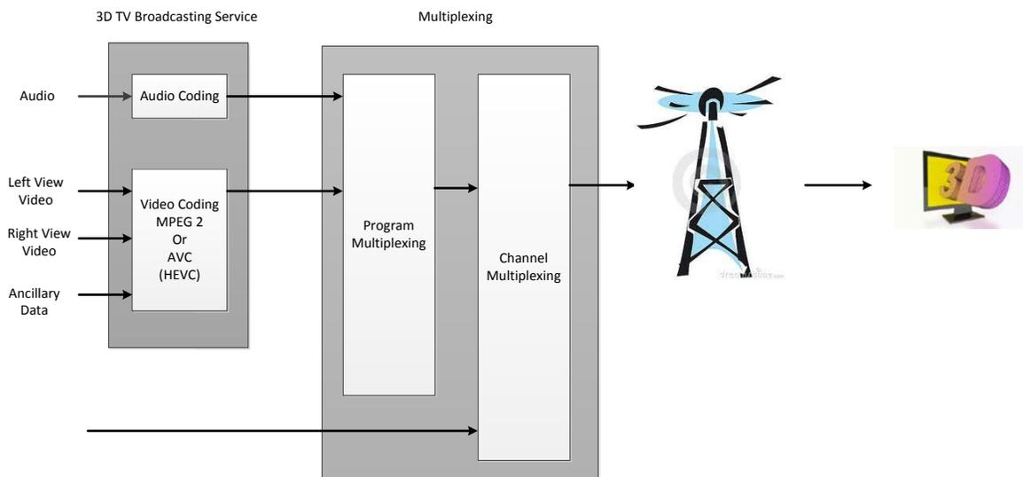
**Figure 1.1** Frame Compatible 3D Broadcasting System.
