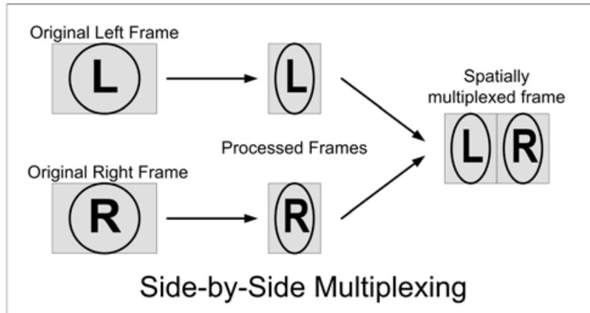
**Figure 5.4** Side-by-Side Multiplexing<sup>4</sup>.
