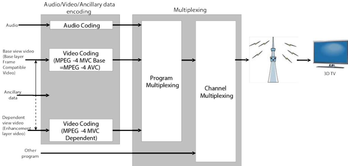
**Figure 1.2** Multi-Resolution Frame Compatible 3D Broadcasting System.
